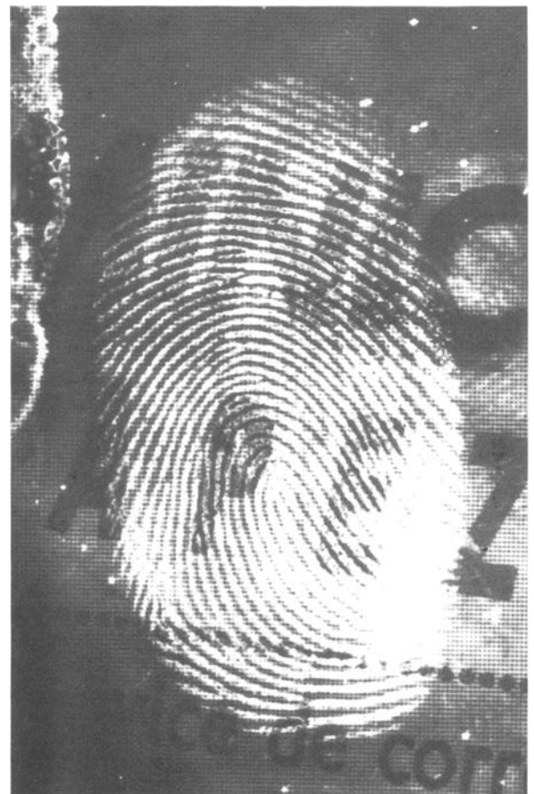
FIG. 7—Cyanoacrylate print developed on a multicolored plastic credit card dyed by EuTTAPhen.
